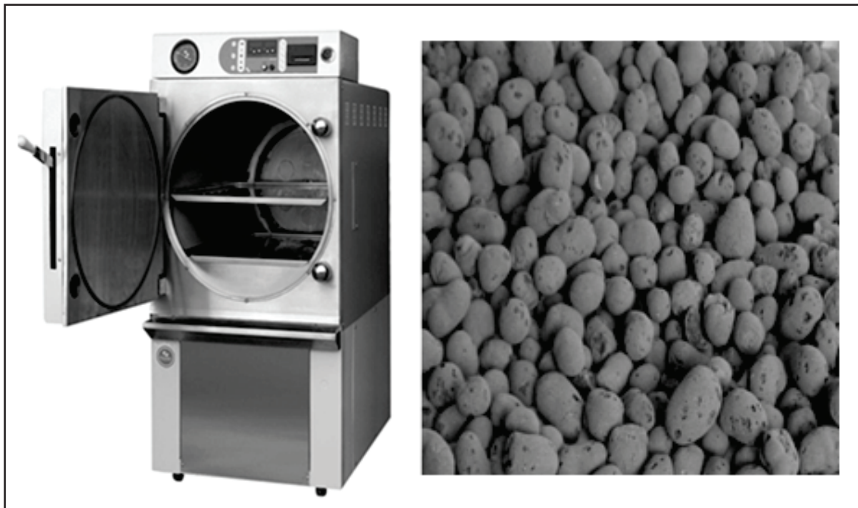
Fig. 3. Autoclave Machine and Autoclaved Fly-ash Pellet
