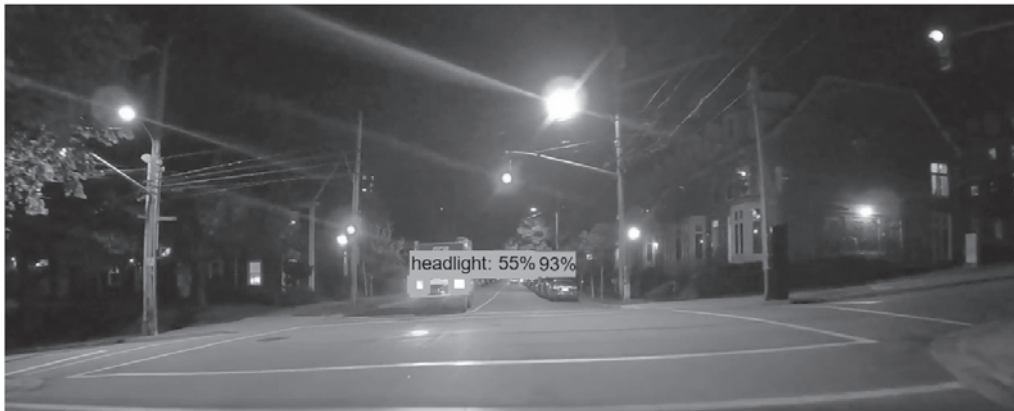
Fig. 1. Detection of Headlights With Background Lights
