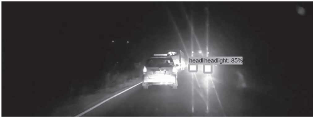
Fig. 3. Detection of Headlights Ignoring Tail Lights
