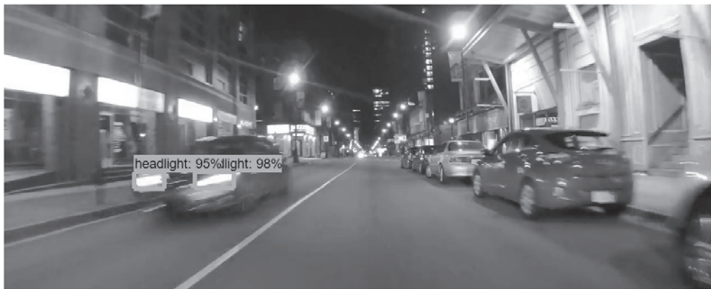
Fig. 2. Detection of Headlights With Background Noise
