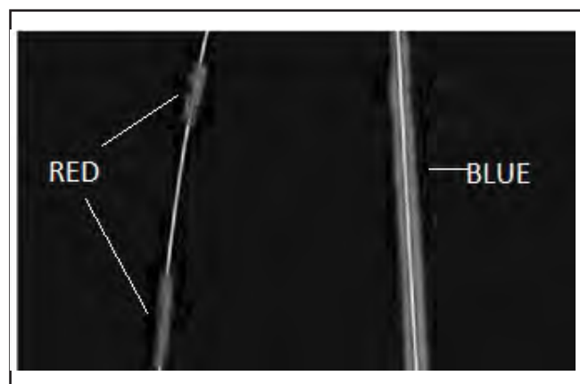
Fig. 3. Detecting Lane Lines With Sliding Windows
